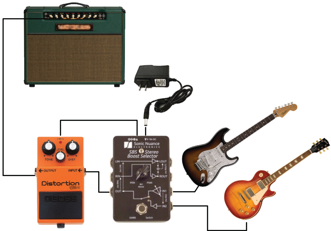
Figure A: AB switch with boost and DC output driving another effect. In this scenario the stereo signal path is left unused.
