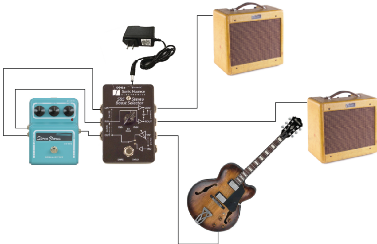
Figure B: Foot switchable boost with Stereo buffering and ground isolation. Guitar signal sent to stereo chorus effect. Stereo output sent to two outputs with transformer isolation on LOUT.
